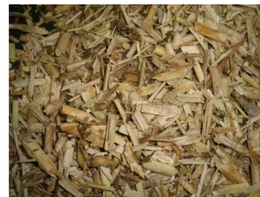
Kenaf insulation ( \lambda=0,036 - 0,039 W/mk)
